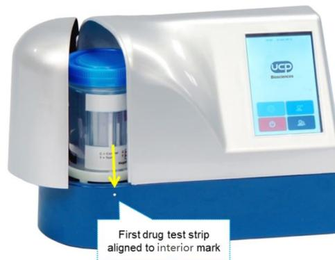
Fig5: Reader station. The mark is a white dot on the blue base.
